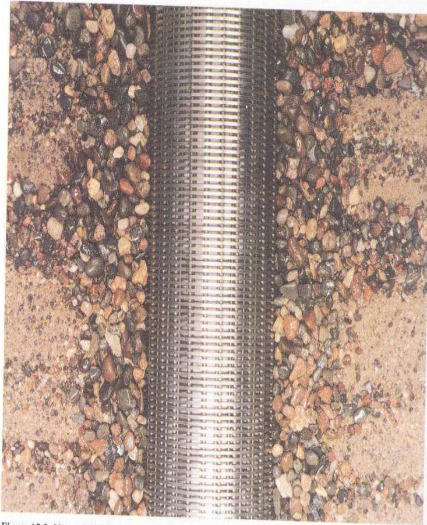
Figure 15.3. Natural development removes most particles near the well screen that are smaller than the slot openings, thereby increasing porosity and hydraulic conductivity in a zone surrounding the screen.
